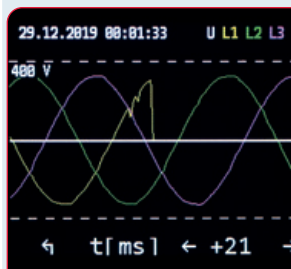
Graphical diagnosis of voltage and current history in case of a voltage dip according to IEC 61000-4-30
